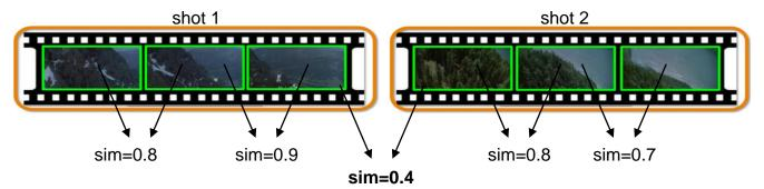
In the example above, there are two shots each with 3 frames, and we are given the similarity values between subsequent frames. As we see, the similarity value of the two frames at boundary of the shots is much smaller than the ones between frames within a shot. If we use a threshold, for example, of 0.5, we can safely detect the shot segmentation.
