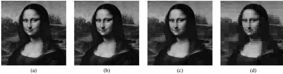
**Figure 9**  $L^2$  wavelet image compression: The original image (a) can be represented using (b) 19% of its wavelet coefficients, with 5% relative  $L^2$  error; (c) 3% of its coefficients, with 10% relative  $L^2$  error; and (d) 1% of its coefficients, with 15% relative  $L^2$  error.
