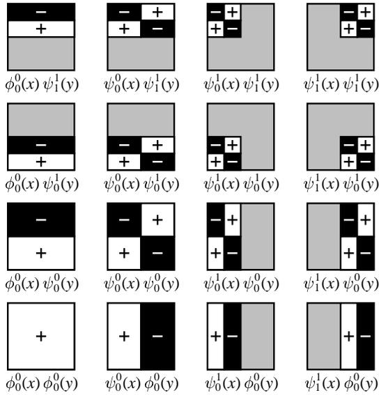
**Figure 7** Standard construction of a two-dimensional Haar wavelet basis for  $V^2$ . In the unnormalized case, functions are +1 where plus signs appear, -1 where minus signs appear, and 0 in gray regions.
