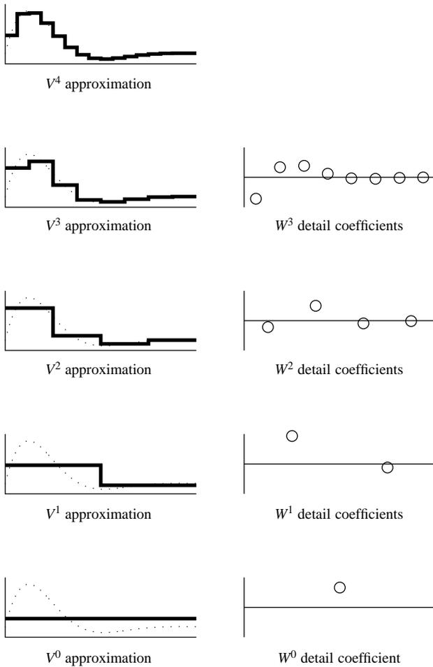
**Figure 1** A sequence of decreasing-resolution approximations to a function (left), along with the detail coefficients required to recapture the finest approximation (right). Note that in regions where the true function is close to being flat, a piecewise-constant approximation works well, so the corresponding detail coefficients are relatively small.
